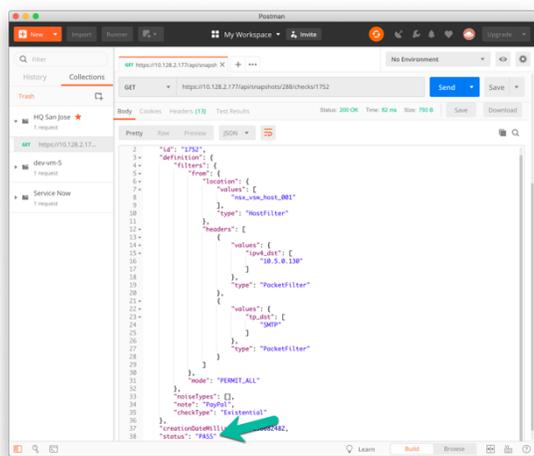
Additionally, Forward Search supports a “permit all mode” function that ignores firewall rules and access lists completely, identifying if the firewall is blocking the traffic, or if the network doesn’t have the appropriate routing or switching infrastructure in place.
